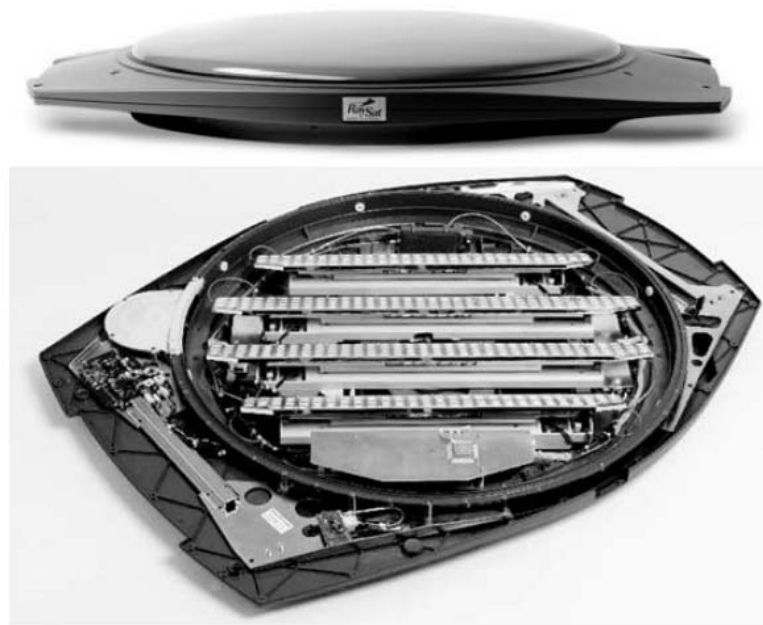
Figure 6.15 Raysat Speedway 1000 hybrid electronically/mechanically steered ultralow profile Ku-band antenna array for mobile TV reception.
