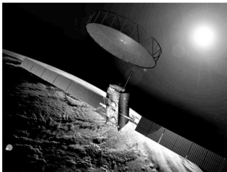
Figure 6.9 Artist's impression of the Inmarsat-4 satellite with its 9 m Astromesh reflector unfurled.
