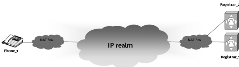
Figure 11.10 Proxy server and registrar behind the same NAT box
